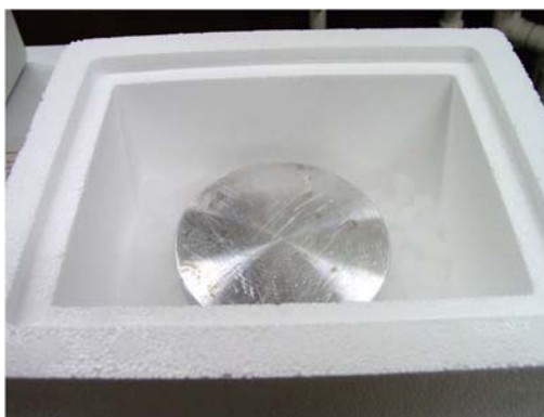
Fig. 3 Aluminum disc, approximately 125 mm in diameter \times 15 mm, on dry ice inside a Styrofoam shipping carton.
