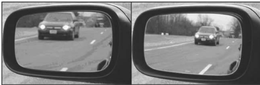
Figure 2. The view in flat ( left ) versus convex ( right ) driver-side mirrors. Image detail from Wierwille et al. (2008).
